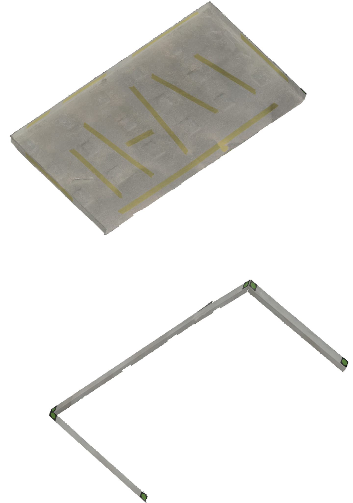
complete and partial scans of balcony element
